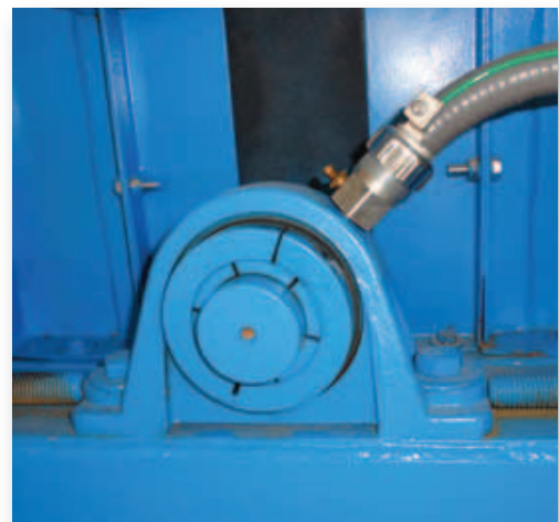
TT420Z-LT installed in a pillow-block bearing.
